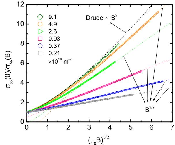
**Fig. 2.** (Color online) Normalized inverse-magnetoconductivity plotted as a function of  $(\mu_0 B)^{3/2}$  at  $T = 1.22$  K.
