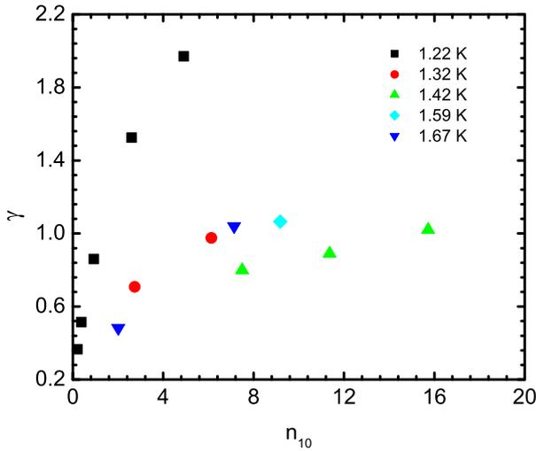
**Fig. 3.** (Color online) The parameter  $\gamma$  versus density at various temperatures.
