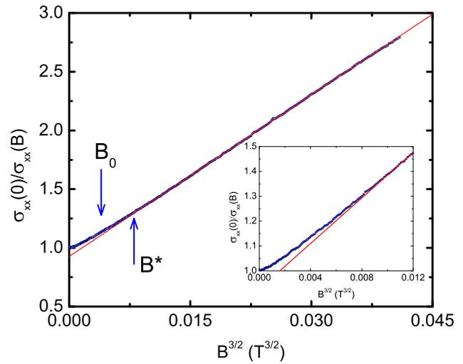
**Fig. 1.** (Color online) Normalized inverse magnetoconductivity vs  $B^{3/2}$  for  $n_{10} = 0.21$ . The definition of  $B^*$ , denoted by an arrow, is defined below. The inset is a blow-up of the plot in the low field region. The solid line is a qualitative fit given by Eq. (4).
