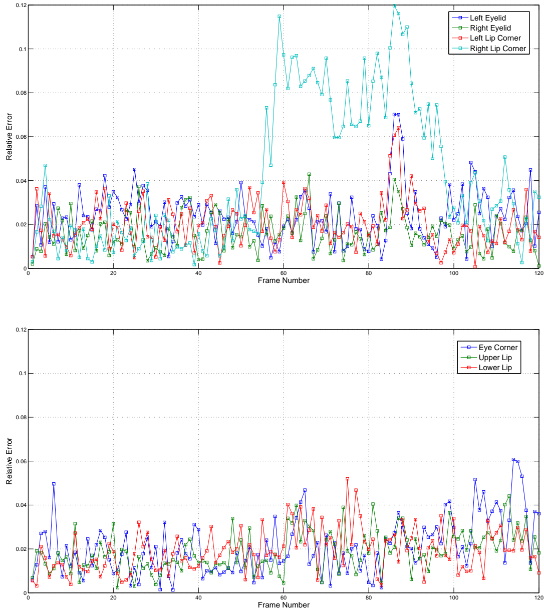
Fig. 9: Tracking error for significant facial features. The pixel error for each feature is divided by the approximate width of the face in pixels. Top: Frontal features. Bottom: Profile features.
