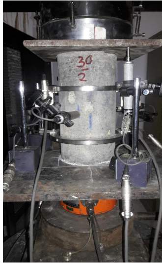
Figure 3.12: Uniaxial compressive Cylindrical test setup and measuring instruments
