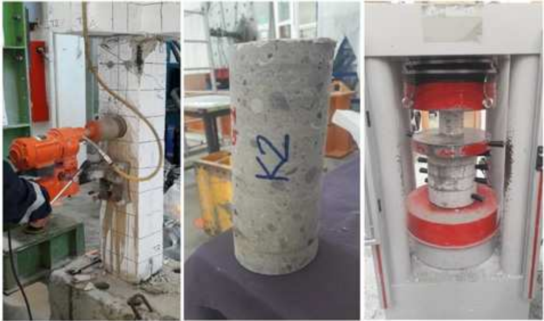
Figure 3.12: Drilling and testing of core specimens
