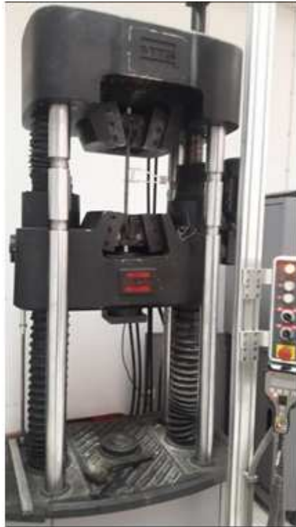
Figure 3.16: Test setup for longitudinal reinforcement
