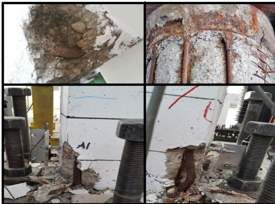
Figure 2.1: Natural corrosion process and cover concrete cracking.
