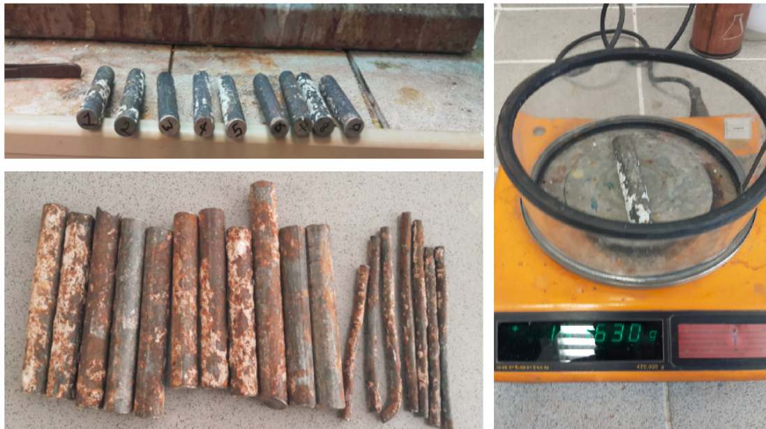
Figure 4.27: Corroded bars and cleaning process by special solution.
