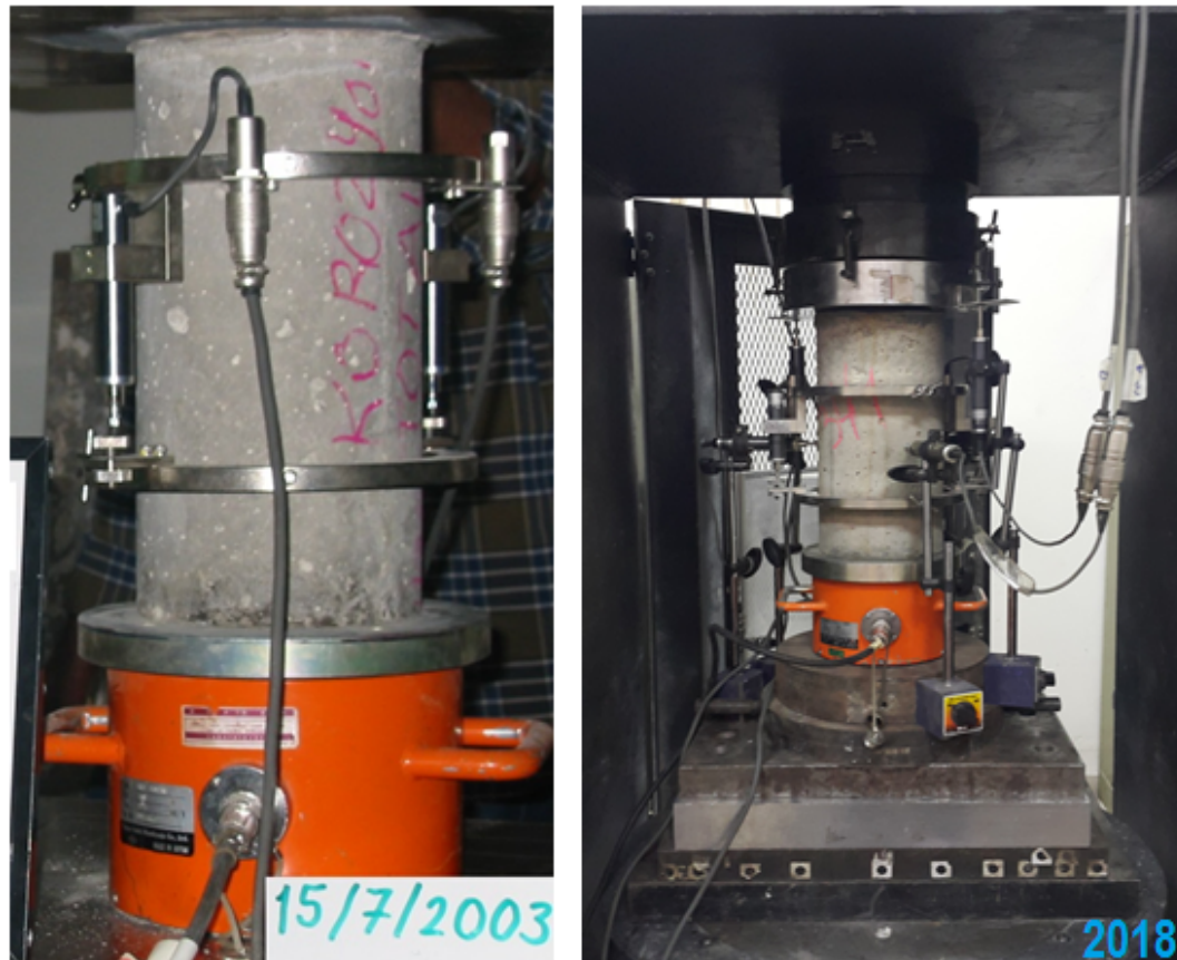
Figure 4.13: Standard cylinder specimen tests 28th days and 5420th days.
