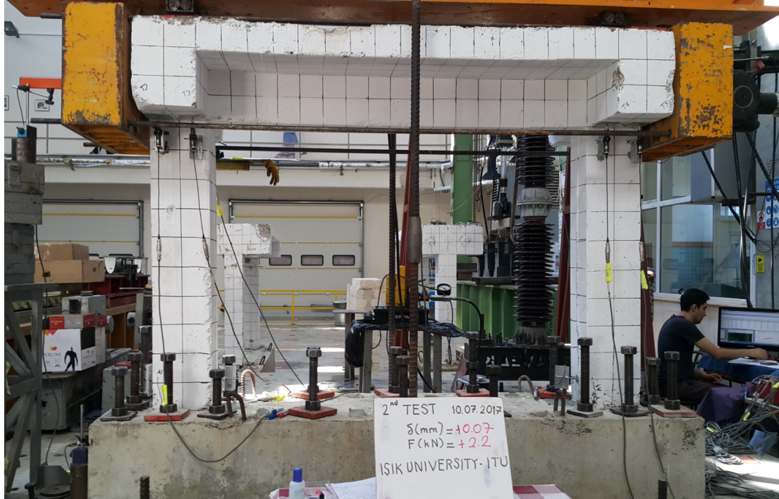
Figure 4.9: LVDTs connected and 2 nd step (+0.07 mm) of the experiment achieved.
