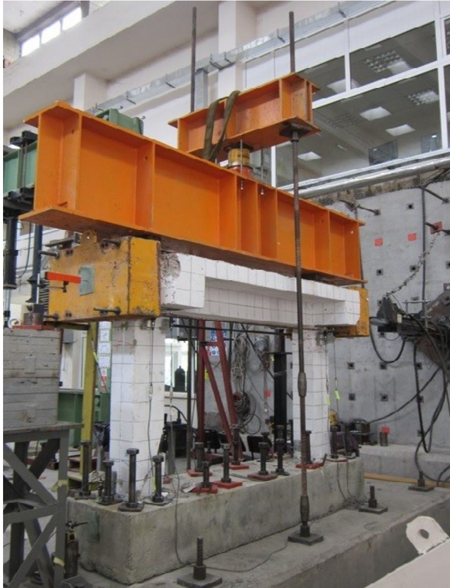
Figure 4.8: Test setup of the experimental works.
