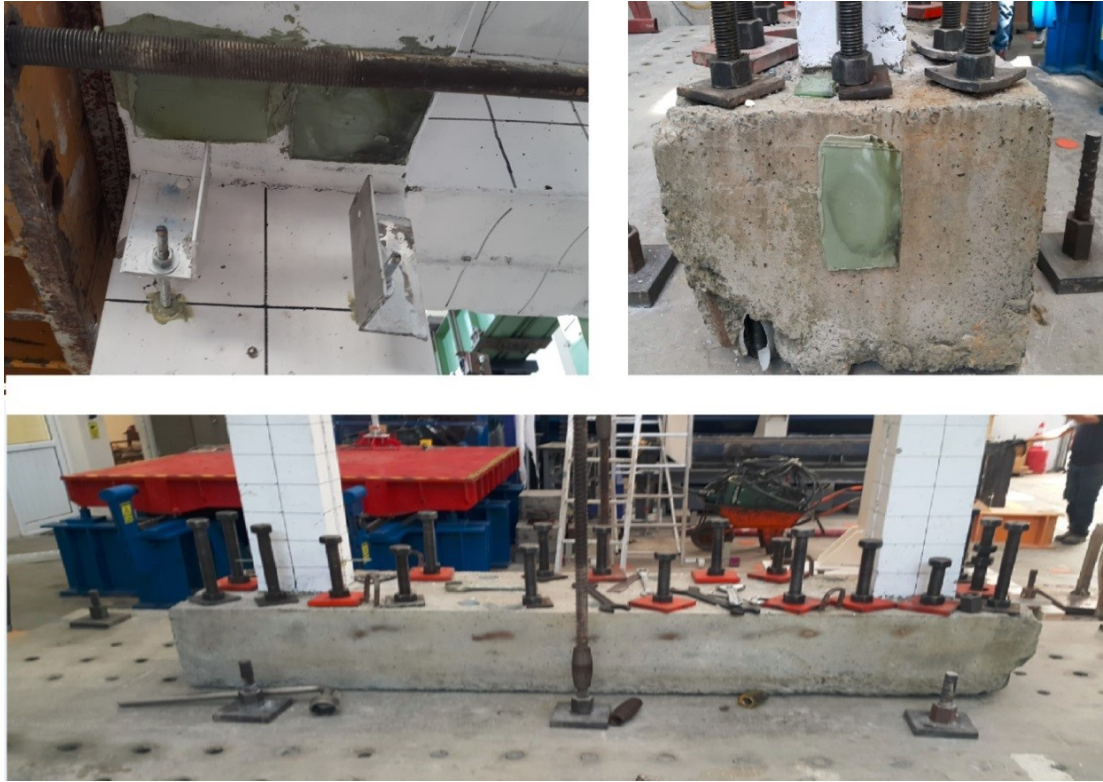
Figure 4.7: Preparation of RC Frame specimen for the test: (left) Mirror and holes for LVDTs (right) Mirror for foundation slippage measurement surface (bottom) Anchorage of the specimens to the adaptor ground.
