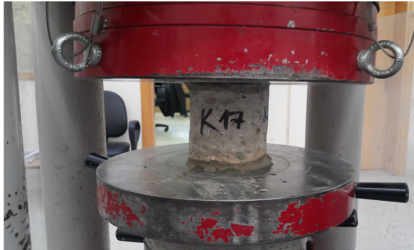
Figure 4.20: Core specimens and testing equipment of press tool.
