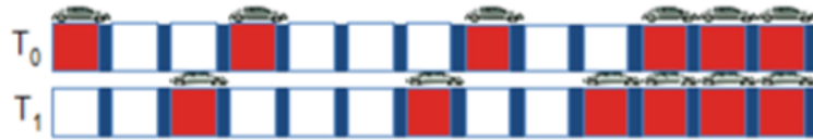
Figure 3.1: Vehicle Propagation based on Cell Automata Traffic Flow Model [20].
