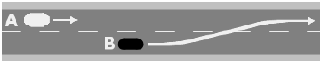
Figure 3.3: Representation of Vehicle A and Vehicle B for understanding Maximum Cooperative Deceleration [63].
