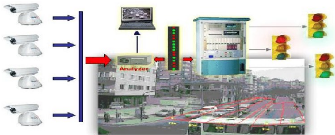
Figure 2.8: An example of Camera Traffic Analysis System [24].
