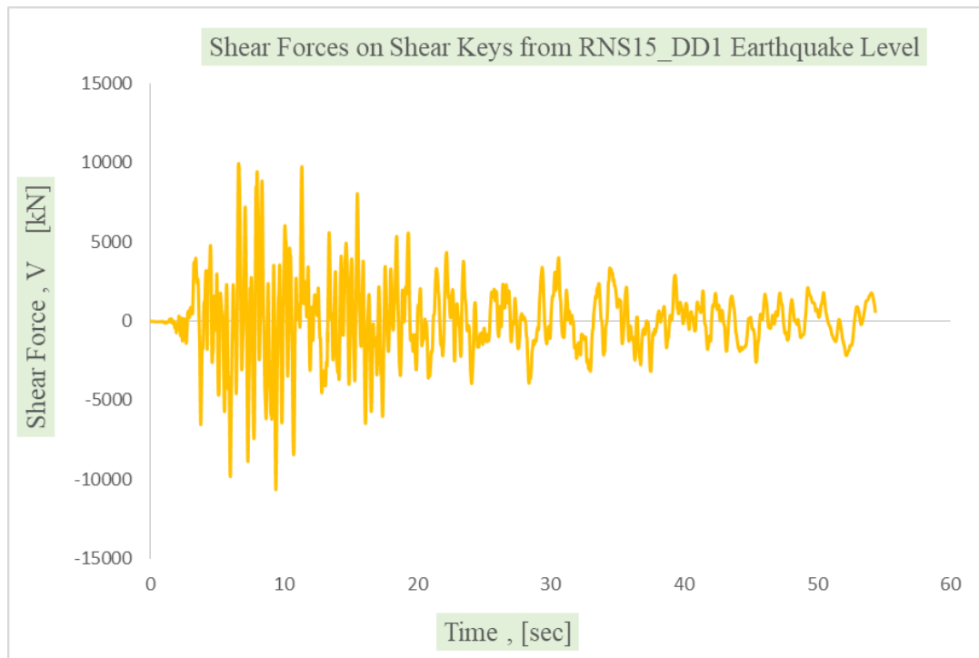
Figure 8.17. Shear Forces on Shear Key at Abutments
