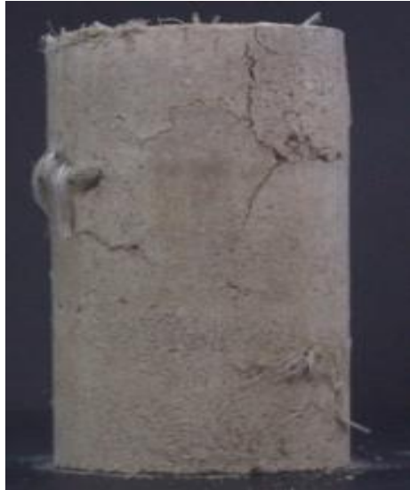
Figure 6.59 Peak point of CH+0.25% polypropylene ( \omega = 24\% , q_u = 254.9 kN/m 2 ) (Etminan, 2012)
