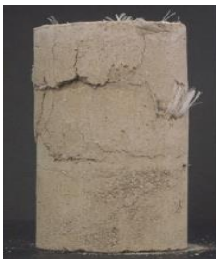
Figure 6.76 Peak point of CH+0.75% polypropylene ( \omega = 25\% , q_u = 317 kN/m 2 ) (Etminan, 2012)
