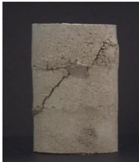
Figure 6.2 Peak point of high plasticity clay soil ( \omega = 27\% , q_u = 174.7 kN/m 2 ) (Etminan, 2012)
