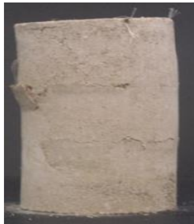
Figure 6.85 Peak point of CH+1% polypropylene ( \omega = 25.7\% , q_u = 315.4 kN/m 2 ) (Etminan, 2012)
