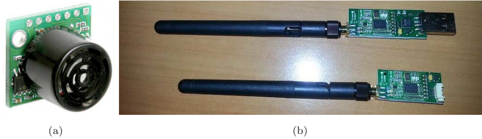
Figure 2.8: (a) Maxbotix LV-MaxSonar-EZ0 Sonar; (b) 3DR radio kit 433MHz
