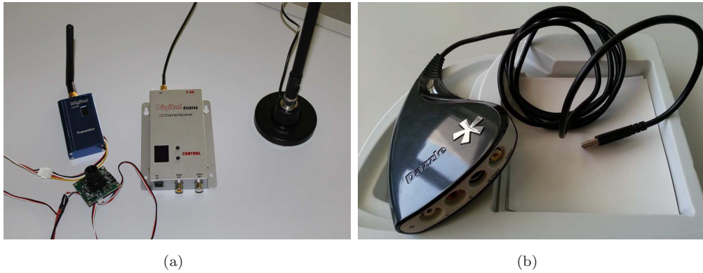
Figure 2.10: (a) 1000mW 2.4GHz video transmitter, 12 channel receiver, 1/3'' CCD camera; (b) Dazzle video capture card
