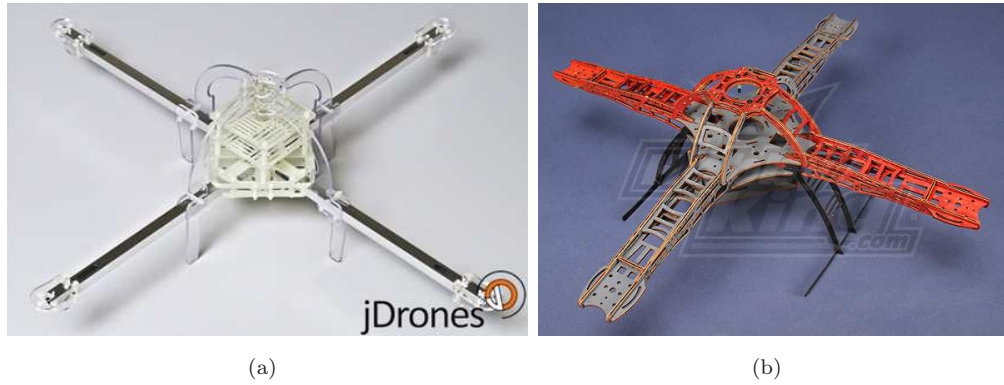
Figure 2.3: Quadcopter frames: (a) Jdrones Arducopter quad frame V1[20]; (b) HobbyKing quadcopter frame V1[21]
