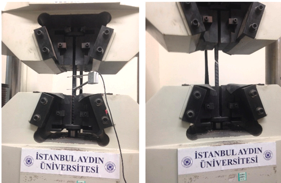
Fig. 8. Tensile test of the rebar.
