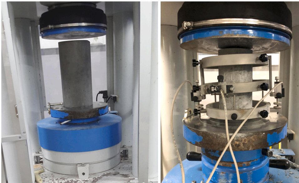
Fig. 7. Compression tests of the concrete samples.
