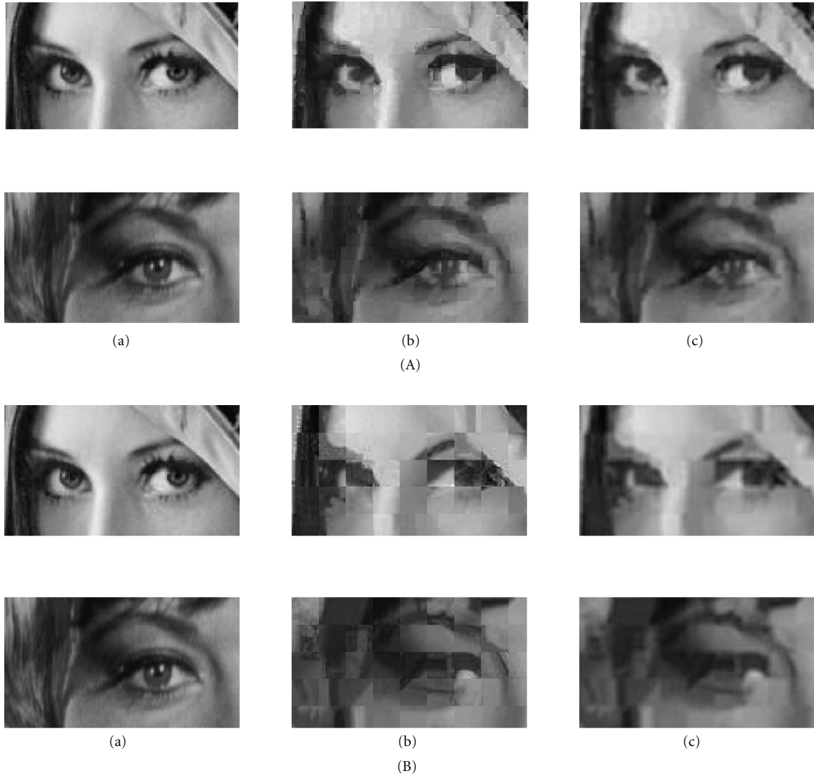
FIGURE 13: (A) Cropped (a) original, (b) reconstructed, and (c) filtered versions of the images (Lenna and F73) for the 1st group of experiments (Fold 1). Lenna: PSNR = 28,93 and 29,66 (filtered), F73: PSNR = 33,36 and 34,11 (filtered) (CR = 21,33). (B) Cropped (a) original, (b) reconstructed, and (c) filtered versions of the images (Lenna and F73) for the 2nd group of experiments. Lenna: PSNR = 25,20 and 25,87 (filtered), F73: PSNR = 29,58 and 30,36 (filtered) (CR = 70,62).
