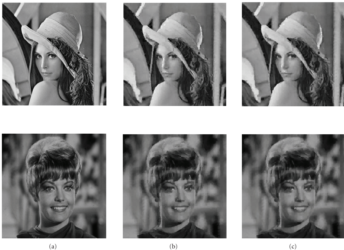
FIGURE 12: (a) Original, (b) reconstructed, and (c) filtered versions of the images (Lenna and F73) for the 2nd group of experiments. Lenna: PSNR = 25,20 and 25,87 (filtered), F73: PSNR = 29,58 and 30,36 (filtered) (CR = 70,62).
