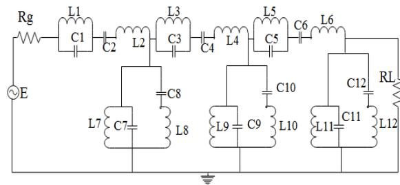
**Figure 9.** Synthesized normalized dual-band filter ( $R_g=1\Omega$ ,  $L_1=0.3139H$ ,  $C_1=0.041F$ ,  $L_2=0.3H$ ,  $C_2=0.043F$ ,  $L_3=1.01H$ ,  $C_3=0.013F$ ,  $L_4=0.95H$ ,  $C_4=0.014F$ ,  $L_5=0.711H$ ,  $C_5=0.018F$ ,  $L_6=0.67H$ ,  $C_6=0.02F$ ,  $L_7=0.0173H$ ,  $C_7=0.738F$ ,  $L_8=0.0162H$ ,  $C_8=0.785F$ ,  $L_9=0.0141H$ ,  $C_9=0.903F$ ,  $L_{10}=0.0133H$ ,  $C_{10}=0.9602F$ ,  $L_{11}=0.0524H$ ,  $C_{11}=0.243F$ ,  $L_{12}=0.05H$ ,  $C_{12}=0.259F$ ,  $R_L=1\Omega$ )
