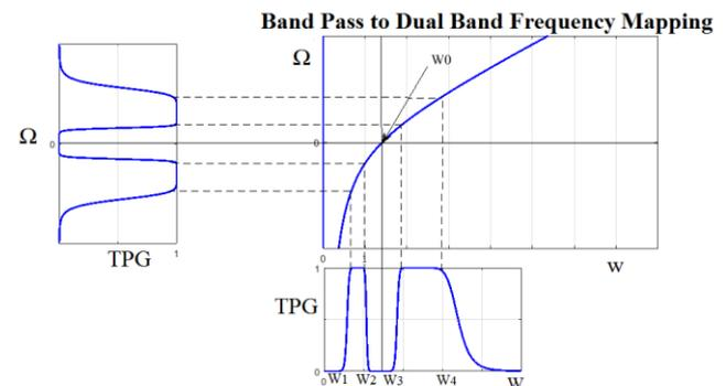
Figure 6. Band-pass to dual-band frequency mapping
