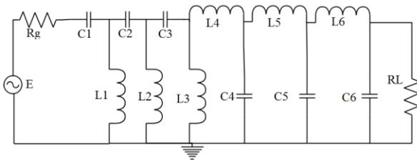
**Figure 11.** Synthesized normalized BP prototype ( $R_g=1\Omega, L_1=0.816H, C_1=1.63F, L_2=0.72H, C_2=0.68F, L_3=2.05H, C_3=0.86F, L_4=0.66H, C_4=0.65F, L_5=1.72H, C_5=0.67F, L_6=1.03H, C_6=0.42F, R_L=1\Omega$ )
