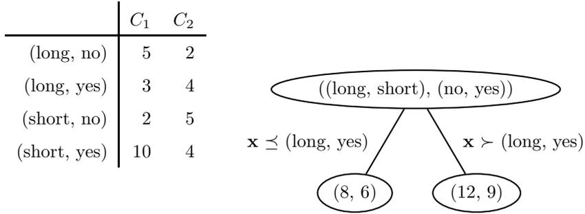
Figure 5: An example case for calculating the impurity of a 2-ordered split. Given the 2-ordering  $((\text{long}, \text{short}), (\text{no}, \text{yes}))$ , the impurity of the split  $\mathbf{x} \preceq (\text{long}, \text{yes})$  will be calculated from the counts of the left branch ( $N_1^L = 8, N_2^L = 6$ ) and right branch ( $N_1^R = 12, N_2^R = 9$ ).
