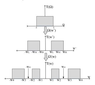
Figure 1. Low pass to dual-band transformation
