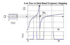
Figure 2. Low-pass to dual-band frequency mapping
