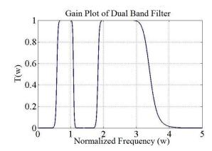
Figure 10. Filter TPG response of Example 1
