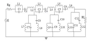
Figure 9. Synthesized normalized dual-band filter (Rg=1Ω, L1=0.3139H, C1=0.041F, L2=0.3H, C2=0.043F, L3=1.01H, C3=0.013F, L4=0.95H, C4=0.014F, L5=0.711H, C5=0.018F, L6=0.67H, C6=0.02F, L7=0.0173H, C7=0.738F, L8=0.0162H, C8=0.785F, L9=0.0141H, C9=0.903F, L10=0.0133H, C10=0.9602F, L11=0.0524H, C11=0.243F, L12=0.05H, C12=0.259F, RL=1Ω)
