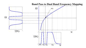
Figure 6. Band-pass to dual-band frequency mapping
