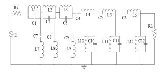
Figure 12. Synthesized normalized dual-band filter (Rg=1 $\Omega$ , L1=0.0167H, C1=0.7617F, L2=0.0401H, C2=0.318F, L3=0.0317H, C3=0.402F, L4=0.3084H, C4=0.0413F, L5=0.8037H, C5=0.016F, L6=0.4813H, C6=0.0265F, L7=0.3813H, C7=0.0334F, L8=0.3364H, C8=0.038F, L9=0.958H, C9=0.0133F, L10=0.042H, C10=0.304F, L11=0.0407H, C11=0.3131F, L12=0.065H, C12=0.1963F, RL=1 $\Omega$ )
