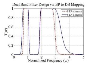
**Figure 14.** Filter response generated by BP to DB approach with different number of LP elements in BP prototype
