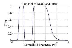
Figure 13. Filter TPG response of Example 2
