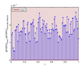
Figure 6. Difference between the the exact solution and 2nd order Tikhonov solution for g(0.625, t) of problem (1.5) with noisy data when  $\Delta t = 0.01$ .
