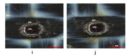
FIGURE 1. Optical microscope images of cavities obtained with (a) and (b) 0.1 J pulse energy, (c) and (d) 1 J pulse energy, (e) and (f) 2 J pulse energy, (g) and (h) 3 J pulse energy, (i) and (j) 4 J pulse energy.
