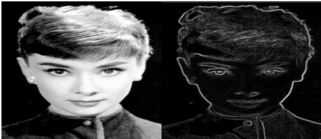
Figure 5.14: Result of the gradient command. (a) original image, (b) result image
